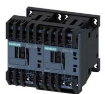
reversing contactor assembly, AC-3e/AC-3, 9 A, 4 kW / 400 V, 3-pole, 110 V AC, 50/60 Hz, spring-loaded terminal, electrical and mechanical interlock
