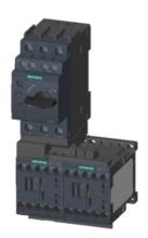
Fuseless motor starter Reversing operation 600VAC Size S00 4.5-6.3A 24V DC screw connection For screw mounting Or 35 mm rail-mounting Type of coordination 1 1NO+1NC (MSP) 1NC (per contactor)
