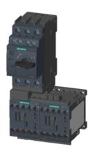
Fuseless motor starter Reversing operation 600VAC Size S00 0.55-0.8A 24V DC screw connection For screw mounting Or 35 mm rail-mounting Type of coordination 2 IQ = 150 KA Also full fills type Of coordination 1 1NO+1NC (MSP) 1NC (per contactor)
