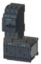
FUSELESS MOTOR STARTER REVERSING OPERATION 600V AC SZ S00 0.11-0.16A 24V DC SCREW CONNECTION FOR SCREW MOUNTING OR 35 MM RAIL-MOUNTING TYPE OF COORDINATION 2 IQ = 150 KA ALSO FULFILLS TYPE OF COORDINATION 1 1NO+1NC (MSP) 1NC (PER CONTACTOR)
