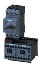
Load feeder fuseless, Reversing duty 400 V AC, Size S00 4.50...6.30 A 24 V DC screw terminal for installation on standard mounting rail Type of coordination 1, Iq = 150 kA 1 NC (contactor)
