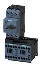
Load feeder fuseless, Reversing duty 400 V AC, Size S00 3.50...5.00 A 24 V DC screw terminal for installation on standard mounting rail Type of coordination 1, Iq = 150 kA 1 NC (contactor)
