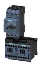
Load feeder fuseless, Reversing duty 400 V AC, Size S00 1.10...1.60 A 230 V AC screw terminal for installation on standard mounting rail (also fulfills type of coordination 1) Type of coordination 2, Iq = 150 kA 1 NC (contactor)
