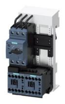
Load feeder fuseless, Reversing duty 400 V AC, Size S00 0.55...0.80 A 230 V AC screw terminal for 60 mm busbar systems (also fulfills type of coordination 1) Type of coordination 2, Iq = 150 kA 1 NC (contactor)
