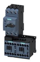
Load feeder fuseless, Reversing duty 400 V AC, Size S00 0.55...0.80 A 230 V AC screw terminal for installation on standard mounting rail (also fulfills type of coordination 1) Type of coordination 2, Iq = 150 kA 1 NC (contactor)
