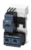
Load feeder fuseless, Reversing duty 400 V AC, Size S00 0.45...0.63 A 24 V DC screw terminal for 60 mm busbar systems (also fulfills type of coordination 1) Type of coordination 2, Iq = 150 kA 1 NC (contactor)
