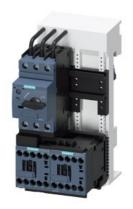
Load feeder fuseless, Reversing duty 400 V AC, Size S00 0.45...0.63 A 230 V AC screw terminal for 60 mm busbar systems (also fulfills type of coordination 1) Type of coordination 2, Iq = 150 kA 1 NC (contactor)
