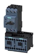
FUSELESS LOAD FEEDER REVERSING OPERATION, 400 V AC, S00 0.45 TO 0.63 A 3 KW, 110/120V AC 50/60 HZ SCREW TERMINAL FOR STANDARD RAIL MOUNTING, TYPE OF COORDINATION 2, IQ = 150 KA (ALSO FULFILLS TYPE OF COORDINATION 1) 1NC (CONTACTOR)
