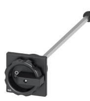
Door-coupling rotary operating mechanism black 66x66 mm, Front plate mounting Central hole mounting 22.5mm with coupling part with shaft 300 mm long, 6x6 mm, accessories for load disconnector 3LD3
