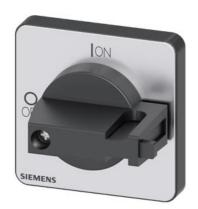
selector switch, black 48x48 mm Front plate mounting Central hole mounting 22.5mm for shaft 6x6 mm, accessory for Load disconnector 3LD3
