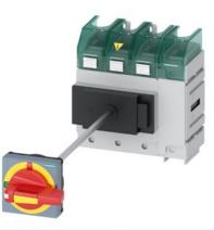
SENTRON, Molded case switch 3LD5 UL, Emergency switching-off, 4-pole, certified according to UL489 UL60947-4-1 and IEC60947-3, UL: 125A, SCCR 65kA at 480VAC, Operating power at 480VAC 3-phase: 75hp, IEC: 125A, Operating power at AC-23A at 400V: 55kW, floor mounting with door coupling rotary operating mechanism, defeatable, emergency switching-off, 4-hole mounting of the handle, without tolerance compensation, incl. terminal covers for the infeed side
