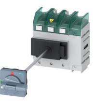
SENTRON, Molded case switch 3LD5 UL, Main switch, 4-pole, certified according to UL489 UL60947-4-1 and IEC60947-3, UL: 125A, SCCR 65kA at 480VAC, Operating power at 480VAC 3-phase: 75hp, IEC: 125A, Operating power at AC-23A at 400V: 55kW, floor mounting with door coupling rotary operating mechanism, defeatable, Standard, 4-hole mounting of the handle, without tolerance compensation, incl. terminal covers for the infeed side
