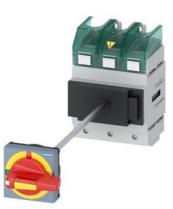
SENTRON, Molded case switch 3LD5 UL, Emergency switching-off, 3-pole, certified according to UL489 UL60947-4-1 and IEC60947-3, UL: 125A, SCCR 65kA at 480VAC, Operating power at 480VAC 3-phase: 75hp, IEC: 125A, Operating power at AC-23A at 400V: 55kW, floor mounting with door coupling rotary operating mechanism, defeatable, emergency switching-off, 4-hole mounting of the handle, without tolerance compensation, incl. terminal covers for the infeed side
