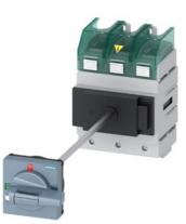
SENTRON, Molded case switch 3LD5 UL, Main switch, 3-pole, certified according to UL489 UL60947-4-1 and IEC60947-3, UL: 125A, SCCR 65kA at 480VAC, Operating power at 480VAC 3-phase: 75hp, IEC: 125A, Operating power at AC-23A at 400V: 55kW, floor mounting with door coupling rotary operating mechanism, defeatable, Standard, 4-hole mounting of the handle, without tolerance compensation, incl. terminal covers for the infeed side
