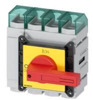
SENTRON, Molded case switch 3LD5 UL, Emergency switching-off, 4-pole, certified according to UL489 UL60947-4-1 and IEC60947-3, UL: 100A, SCCR 65kA at 480VAC, Operating power at 480VAC 3-phase: 60hp, IEC: 100A, Operating power at AC-23A at 400V: 45kW, front-mounted, rotary operating mechanism, red/yellow, 4-hole mounting of the handle, incl. terminal covers for the infeed side
