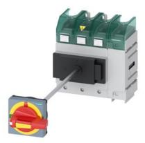
SENTRON, Molded case switch 3LD5 UL, Emergency switching-off, 4-pole, certified according to UL489 UL60947-4-1 and IEC60947-3, UL: 100A, SCCR 65kA at 480VAC, Operating power at 480VAC 3-phase: 60hp, IEC: 100A, Operating power at AC-23A at 400V: 45kW, floor mounting with door coupling rotary operating mechanism, defeatable, emergency switching-off, 4-hole mounting of the handle, without tolerance compensation, incl. terminal covers for the infeed side
