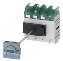
SENTRON, Molded case switch 3LD5 UL, Main switch, 4-pole, certified according to UL489 UL60947-4-1 and IEC60947-3, UL: 100A, SCCR 65kA at 480VAC, Operating power at 480VAC 3-phase: 60hp, IEC: 100A, Operating power at AC-23A at 400V: 45kW, floor mounting with door coupling rotary operating mechanism, defeatable, Standard, 4-hole mounting of the handle, without tolerance compensation, incl. terminal covers for the infeed side
