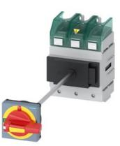
SENTRON, Molded case switch 3LD5 UL, Emergency switching-off, 3-pole, certified according to UL489 UL60947-4-1 and IEC60947-3, UL: 100A, SCCR 65kA at 480VAC, Operating power at 480VAC 3-phase: 60hp, IEC: 100A, Operating power at AC-23A at 400V: 45kW, floor mounting with door coupling rotary operating mechanism, defeatable, emergency switching-off, 4-hole mounting of the handle, without tolerance compensation, incl. terminal covers for the infeed side
