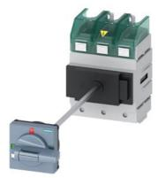
SENTRON, Molded case switch 3LD5 UL, Main switch, 3-pole, certified according to UL489 UL60947-4-1 and IEC60947-3, UL: 100A, SCCR 65kA at 480VAC, Operating power at 480VAC 3-phase: 60hp, IEC: 100A, Operating power at AC-23A at 400V: 45kW, floor mounting with door coupling rotary operating mechanism, defeatable, Standard, 4-hole mounting of the handle, without tolerance compensation, incl. terminal covers for the infeed side
