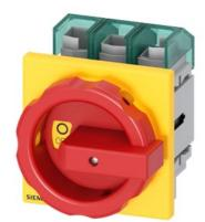
SENTRON, Molded case switch 3LD5 UL, Emergency switching-off, 3-pole, certified according to UL489 UL60947-4-1 and IEC60947-3, UL: 60A, SCCR 50kA at 480VAC, Operating power at 480VAC 3-phase: 40hp, IEC: 63A, Operating power at AC-23A at 400V: 30kW, front-mounted, rotary operating mechanism, red/yellow, 4-hole mounting of the handle, incl. terminal covers for the infeed side
