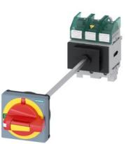
SENTRON, Molded case switch 3LD5 UL, Emergency switching-off, 3-pole, certified according to UL489 UL60947-4-1 and IEC60947-3, UL: 60A, SCCR 50kA at 480VAC, Operating power at 480VAC 3-phase: 40hp, IEC: 63A, Operating power at AC-23A at 400V: 30kW, floor mounting with door coupling rotary operating mechanism, defeatable, emergency switching-off, 4-hole mounting of the handle, without tolerance compensation, incl. terminal covers for the infeed side
