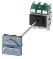
SENTRON 3LD5 switch disconnector UL, main switch, 3-pole, approved according to UL 489, UL 60947-4-1 and IEC 60947-3, UL: 60 A, SCCR 50 kA at 480 V AC, operational power @ 480 V AC 3-phase: 40 hp, IEC: 63 A, operational power at AC-23 A at 400 V: 30 kW, floor mounting with door coupling, defeatable rotary operating mechanism, standard, 4-hole mounting of the handle, without tolerance compensation, including terminal covers for the infeed side for the infeed side
