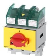
SENTRON, Molded case switch 3LD5 UL, Emergency switching-off, 3-pole, certified according to UL489 UL60947-4-1 and IEC60947-3, UL: 60A, SCCR 50kA at 480VAC, Operating power at 480VAC 3-phase: 40hp, IEC: 63A, Operating power at AC-23A at 400V: 30kW, floor mounting with direct handle, red/yellow, incl. terminal covers for the infeed side
