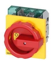
SENTRON, Molded case switch 3LD5 UL, Emergency switching-off, 4-pole, certified according to UL489 UL60947-4-1 and IEC60947-3, UL: 30A, SCCR 50kA at 480VAC, Operating power at 480VAC 3-phase: 20hp, IEC: 32A, Operating power at AC-23A at 400V: 15kW, front-mounted, rotary operating mechanism, red/yellow, 4-hole mounting of the handle, incl. terminal covers for the infeed side
