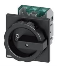
SENTRON 3LD5 switch disconnector UL, main switch, 3-pole, approved according to UL 489, UL 60947-4-1 and IEC 60947-3, UL: 30 A, SCCR 50 kA at 480 V AC, operational power @ 480 V AC 3-phase: 20 hp, IEC: 32 A, operational power at AC-23 A at 400 V: 15 kW, front-mounted: rotary operating mechanism, black, 4-hole mounting of the handle, including terminal covers for the infeed side infeed side
