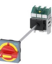
SENTRON, Molded case switch 3LD5 UL, Emergency switching-off, 3-pole, certified according to UL489 UL60947-4-1 and IEC60947-3, UL: 30A, SCCR 50kA at 480VAC, Operating power at 480VAC 3-phase: 20hp, IEC: 32A, Operating power at AC-23A at 400V: 15kW, floor mounting with door coupling rotary operating mechanism, defeatable, emergency switching 4-hole mounting of the handle, without tolerance compensation, incl. terminal covers for the infeed side
