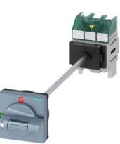
SENTRON, Molded case switch 3LD5 UL, Main switch, 3-pole, certified according to UL489 UL60947-4-1 and IEC60947-3, UL: 30A, SCCR 50kA at 480VAC, Operating power at 480VAC 3-phase: 20hp, IEC: 32A, Operating power at AC-23A at 400V: 15kW, floor mounting with door coupling rotary operating mechanism, defeatable, Standard, 4-hole mounting of the handle, without tolerance compensation, incl. terminal covers for the infeed side
