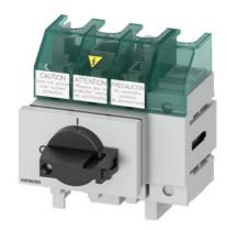
SENTRON, Molded case switch 3LD5 UL, Main switch, 4-pole, certified according to UL489 UL60947-4-1 and IEC60947-3, UL: 30A, SCCR 50kA at 480VAC, Operating power at 480VAC 3-phase: 20hp, IEC: 32A, Operating power at AC-23A at 400V: 15kW, floor mounting with direct handle, black, incl. terminal covers for the infeed side
