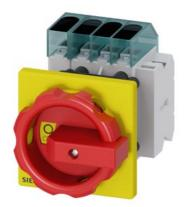
Load disconnector 3LD3, Iu 63 A Main switch 3-pole + N Rated operating capacity at AC-23 A at 400V 22.0 kW Front plate mounting Basic switch with Central hole mounting 22.5mm Toggle drive red / yellow 66x66 mm with auxiliary switch 10E + 1S
