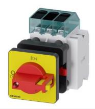
Load disconnector 3LD3, lu 63 A Main switch 3-pole Rated operating capacity at AC-23 A at 400V 22.0 kW Front plate mounting Basic switch with Central hole mounting 22.5mm Toggle drive red / yellow 48x48 mm with auxiliary switch 1OE + 1S
