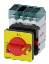
Load disconnector 3LD3, Iu 63 A Main switch 3-pole + N Rated operating capacity at AC-23 A at 400V 22.0 kW Front plate mounting Basic switch with Central hole mounting 22.5mm Toggle drive red / yellow 48x48 mm
