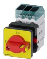
Load disconnector 3LD3, lu 63 A Main switch 3-pole Rated operating capacity at AC-23 A at 400V 22.0 kW Front plate mounting Basic switch with Central hole mounting 22.5mm Toggle drive red / yellow 48x48 mm
