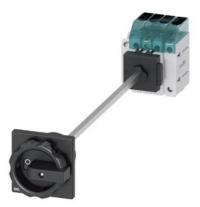
Load disconnector 3LD3, lu 63 A Main switch 3-pole + N Rated operating capacity at AC-23 A at 400V 22.0 kW floor mounting Basic switch with door coupling Central hole mounting 22.5mm Rotating drive black 66 x 66 mm with auxiliary switch 10E + 1S
