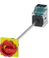
Load disconnector 3LD3, lu 63 A Main switch 3-pole Rated operating capacity at AC-23 A at 400V 22.0 kW floor mounting Basic switch with door coupling Central hole mounting 22.5mm Rotary actuator red / yellow 66 x 66 mm with auxiliary switch 1OE + 1S
