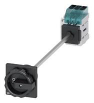
Load disconnector 3LD3, Iu 63 A Main switch 3-pole Rated operating capacity at AC-23 A at 400V 22.0 kW floor mounting Basic switch with door coupling Central hole mounting 22.5mm Rotating drive black 66 x 66 mm with auxiliary switch 10E  $\pm$  1S
