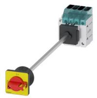
Load disconnector 3LD3, lu 63 A Main switch 3-pole + N Rated operating capacity at AC-23 A at 400V 22.0 kW floor mounting Basic switch with door coupling Central hole mounting 22.5mm Toggle drive red / yellow 48x48 mm with auxiliary switch 10E+1S
