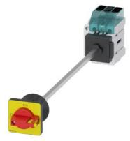
Load disconnector 3LD3, Iu 63 A Main switch 3-pole Rated operating capacity at AC-23 A at 400V 22.0 kW floor mounting Basic switch with door coupling Central hole mounting 22.5mm Toggle drive red / yellow 48x48 mm with auxiliary switch 10E+1S
