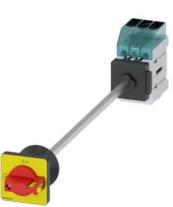
Load disconnector 3LD3, lu 63 A Main switch 3-pole Rated operating capacity at AC-23 A at 400V 22.0 kW floor mounting Basic switch with door coupling Central hole mounting 22.5mm Toggle drive red / yellow 48x48 mm
