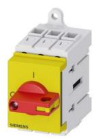
Load disconnector 3LD3, lu 63 A Main switch 3-pole Rated operating capacity at AC-23 A at 400V 22.0 kW Installation in distribution boards, Basic switch with selector knob red / yellow
