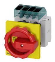
Load disconnector 3LD3, Iu 40 A Main switch 3-pole + N Rated operating capacity at AC-23 A at 400 V 18.5 kW Front plate mounting Basic switch with Central hole mounting 22.5mm Toggle drive red / yellow 66x66 mm with auxiliary switch 10E + 1S
