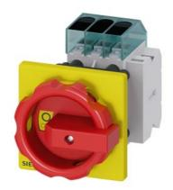
Load disconnector 3LD3, lu 40 A Main switch 3-pole Rated operating capacity at AC-23 A at 400 V 18.5 kW Front plate mounting Basic switch with Central hole mounting 22.5mm Toggle drive red / yellow 66x66 mm with auxiliary switch 1OE + 1S
