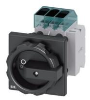
Load disconnector 3LD3, lu 40 A Main switch 3-pole Rated operating capacity at AC-23 A at 400 V 18.5 kW Front plate mounting Basic switch with Central hole mounting 22.5mm Toggle drive black 66x66 mm with auxiliary switch 10E + 1S
