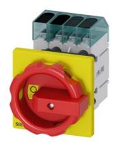
Load disconnector 3LD3, Iu 40 A Main switch 3-pole + N Rated operating capacity at AC-23 A at 400 V 18.5 kW Front plate mounting Basic switch with Central hole mounting 22.5mm Toggle drive red / yellow 66x66 mm
