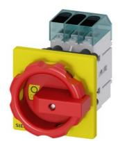
Load disconnector 3LD3, lu 40 A Main switch 3-pole Rated operating capacity at AC-23 A at 400 V 18.5 kW Front plate mounting Basic switch with Central hole mounting 22.5mm Toggle drive red / yellow 66x66 mm
