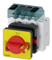
Load disconnector 3LD3, lu 40 A Main switch 3-pole + N Rated operating capacity at AC-23 A at 400 V 18.5 kW Front plate mounting Basic switch with Central hole mounting 22.5mm Toggle drive red / yellow 48x48 mm with auxiliary switch 1OE + 1S
