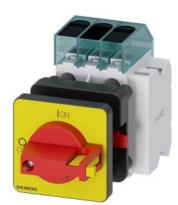
Load disconnector 3LD3, Iu 40 A Main switch 3-pole Rated operating capacity at AC-23 A at 400 V 18.5 kW Front plate mounting Basic switch with Central hole mounting 22.5mm Toggle drive red / yellow 48x48 mm with auxiliary switch 1OE + 1S
